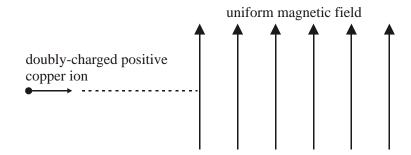
The diagram above shows a doubly-charged positive ion of the copper isotope  $^{63}_{29}$ Cu that is projected into a vertical magnetic field of flux density 0.28 T, with the field directed upwards. The ion enters the field at a speed of  $7.8 \times 10^5$  m s<sup>-1</sup>.
